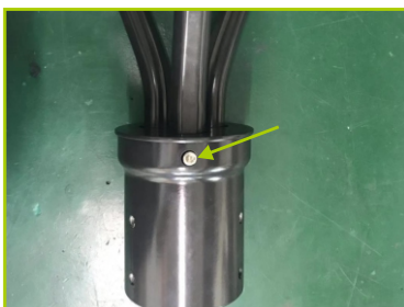
4. Fix the elbow pipes with three M6*12 screws.
